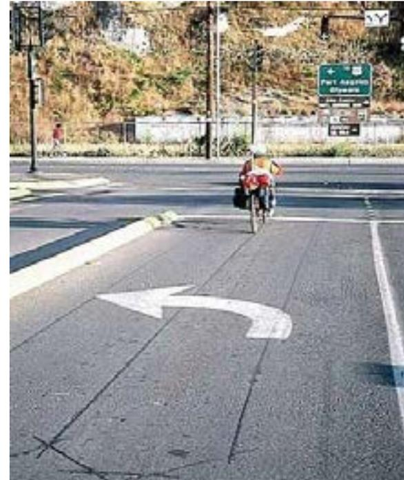
lane. This is the most common type, shown in the photo above. Ride up the middle wire. Usually, there will be a sign and a marking on the pavement indicating where to wait. There may also be diagonal wires, and that works everywhere over the pattern of wires. If there is no middle wire, position your bicycle over one of the side wires, and hope.
