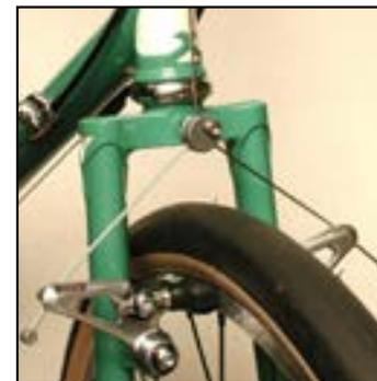
**A traditional cantilever brake without protection for the transverse cable. Tolerable with a smooth tire, but**
