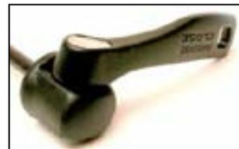
**A Shimano internal-cam quick release**
